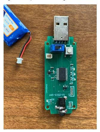
When you look at the connector you will see the black negative wire. The connector is polarized so that goes in with negative wire on the outside edge of the board. It is a locking connector that will snap in.
