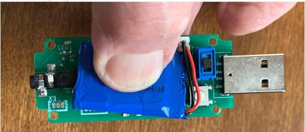
Put the board back in the top casing. Remember the two screws at the USB end
