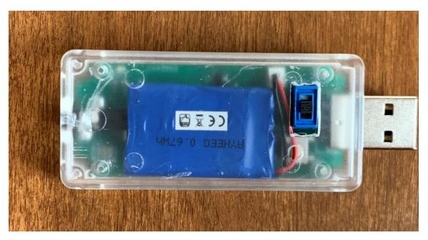
Power it up by moving the 3 position Blue Switch towards the center of the Dongle
