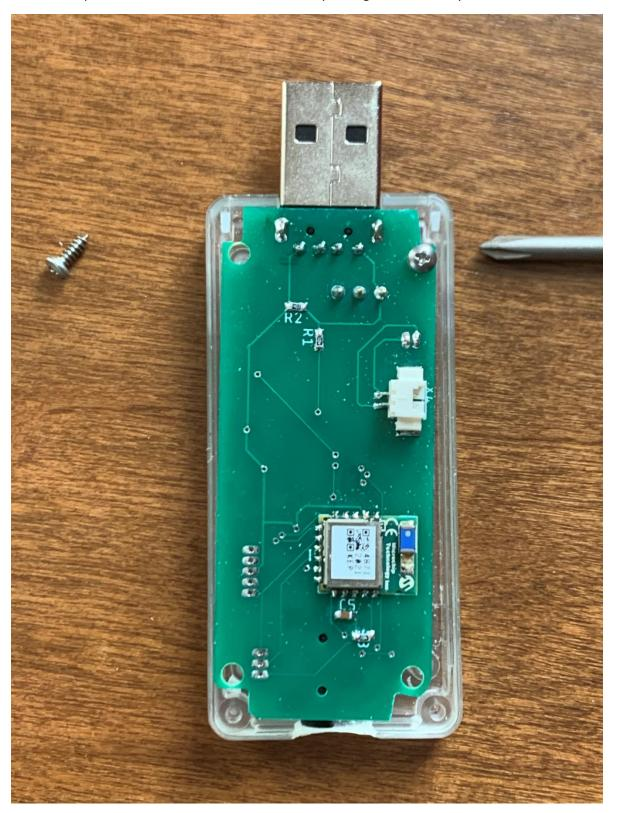
Once the board is out, look at the top of the board. You can see it here with the Hyperion 180 mAH battery. Note the battery socket to the left of the blue switch. This is a Molex Pico Blade connector. The negative is the pin close to the edge of the board.
